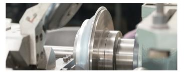
Metal spinning is a type of plastic processing of sheet metal. Formerly called "(drücking)". This method of plastic working uses the susceptibility of materials to deformation (after exceeding the yield point), without breaking the continuity of the shaped sheet. As a result, we obtain from the starting material (e.g. a sheet metal disc) a thin-walled solid of revolution, often of a very complicated shape.
